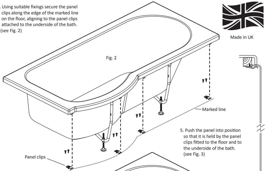
5. Push the panel into position so that it is held by the panel clips fitted to the floor and to the underside of the bath. (see Fig. 3)
